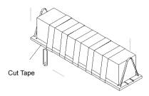
2. Place taped locomotive on a flat surface. Carefully cut the tape along the wood board side surface. Be sure to cut both sides of the wood board. Slowly lift the tape from the locomotive. Be very careful with small parts. Tape cannot be re-used to re-pack the model. Use new packing tape if necessary.
